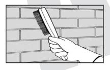
Before using the GPS solution it is important to ensure that the surface onto which it is going is clean and free from dust and loose material and of sufficient integrity and mechanical strength.
