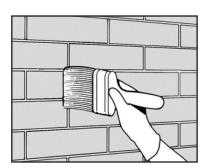
Concrete and masonry surfaces need to be dampened an hour or so before priming (unless already damp, eg, basement walls). Should be damp but surface dry when the primer coat is applied.
