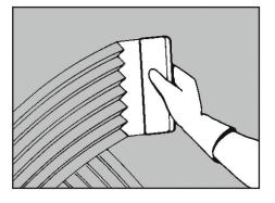
Scratch the surface and leave to set before applying the second coat of similar thickness to the first. For added protection, allow the first coat of render to dry overnight and then apply the second coat of primer. While this is wet and tacky, apply the second coat of render.
